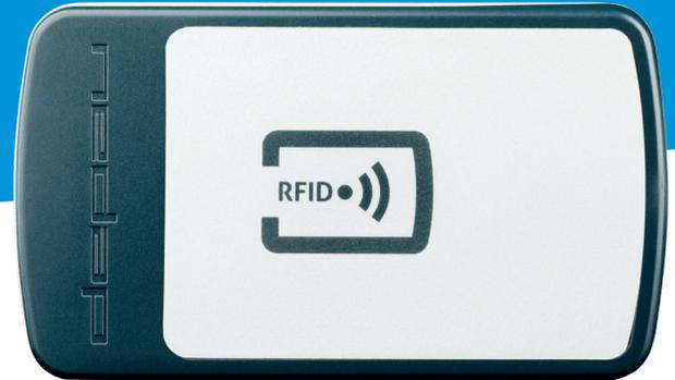
The Window Tag Ultimate is a long-range vehicle identification tag. Based on semi-active RFID technology, the Window Tag Ultimate is identified at distances up to 10 meters (33 feet) with Nedap's TRANSIT Ultimate reader.
